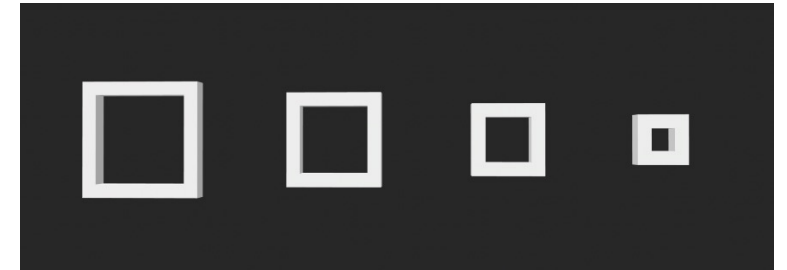
3D Onshape Design: 0.6mm Strut 4mm x 4mm – 1mm x 1mm Pore Array
